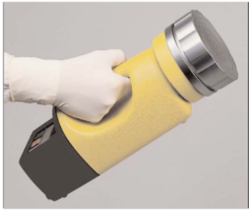
Figure 4.4 - Air Sampler SAS (Surface Air System) Super IAQ model 90593 used for the detection of microbiological contamination of the air
