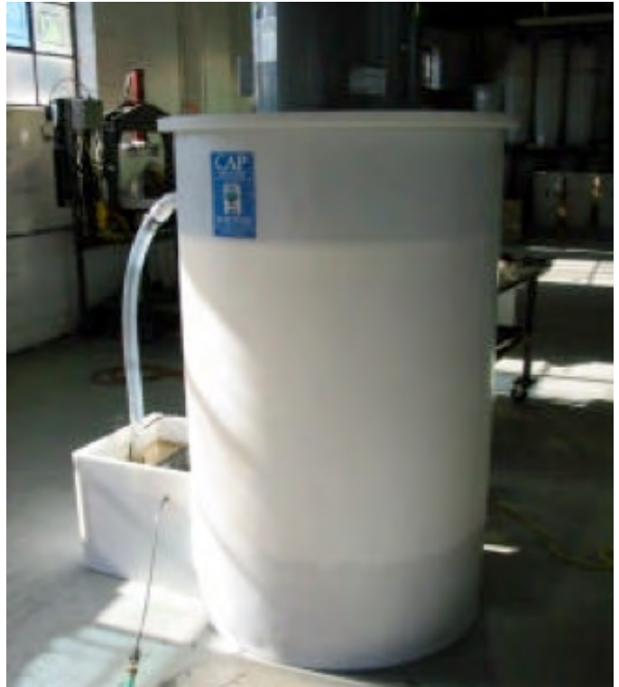
CAP-2500 treats oleoresins and aroma chemicals at a flavor manufacturing process.
